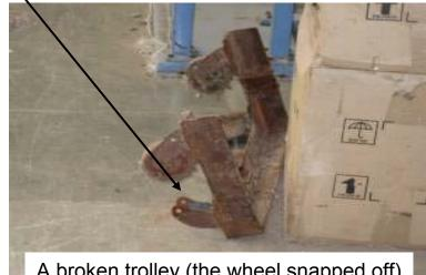
A broken trolley (the wheel snapped off)
