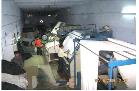
Defects are repaired by hand or cut out from cloth
