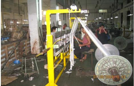
(2) Drawing the warp beam ready for weaving
