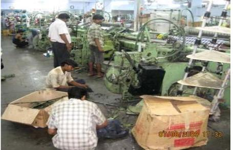
Parts being cleaned and replaced on jammed loom
