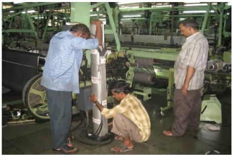
Loom parts being disassembled for diagnosis
