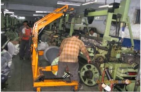
Warp beam being unloaded off a broken loom
