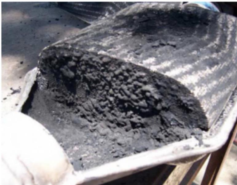
**Figure:** A Diesel Particulate Filter at the End of its Life
