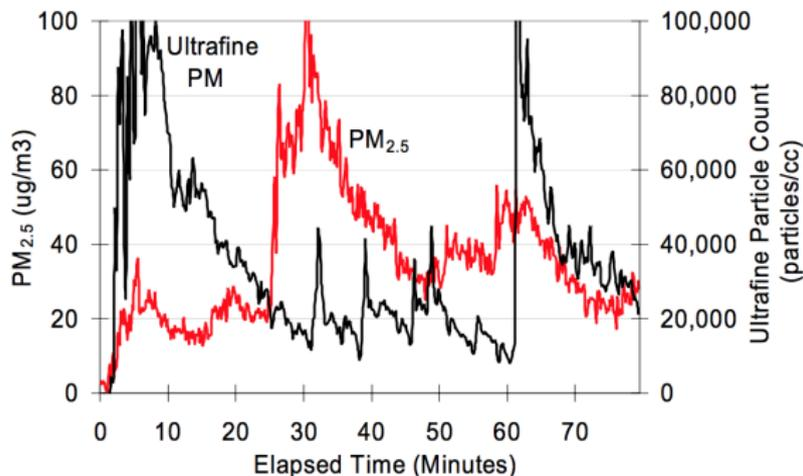
*Figure 1: Conventional buses tested showed significant PM<sub>2.5</sub>, ultrafine particle, black cabin and PAH self-pollution. (Ambient concentrations have been subtracted.)*
