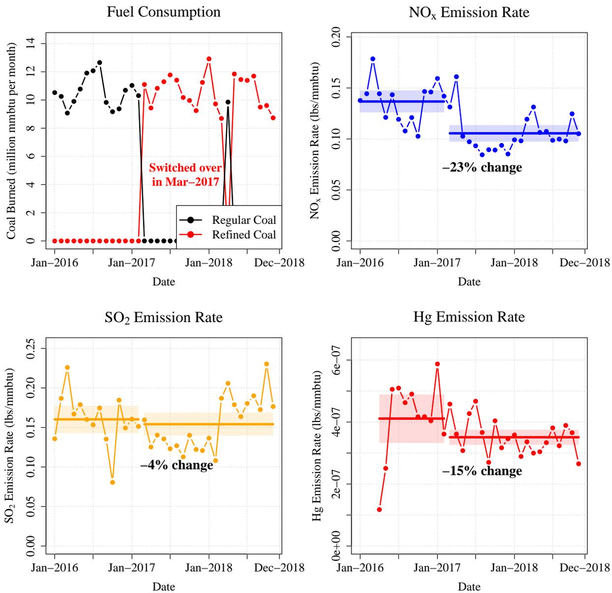
Figure 6: Fuel Consumption and Emission Rates: Plant 3
