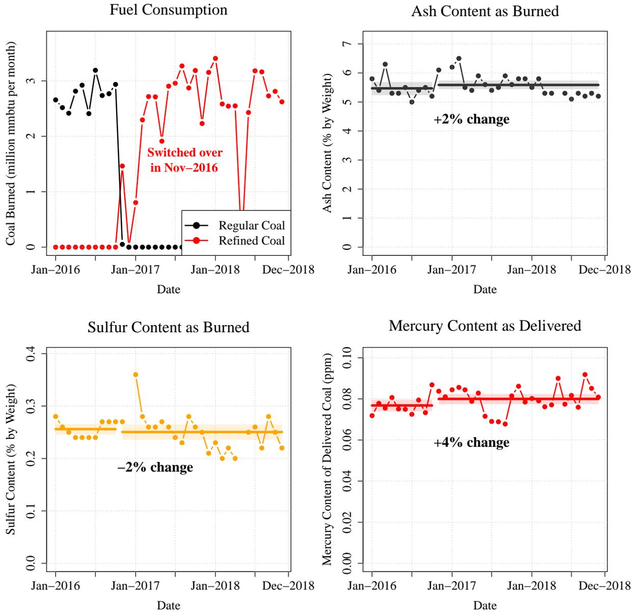
Figure A.2: Coal Characteristics for Plant 1 (in Figure 4)
