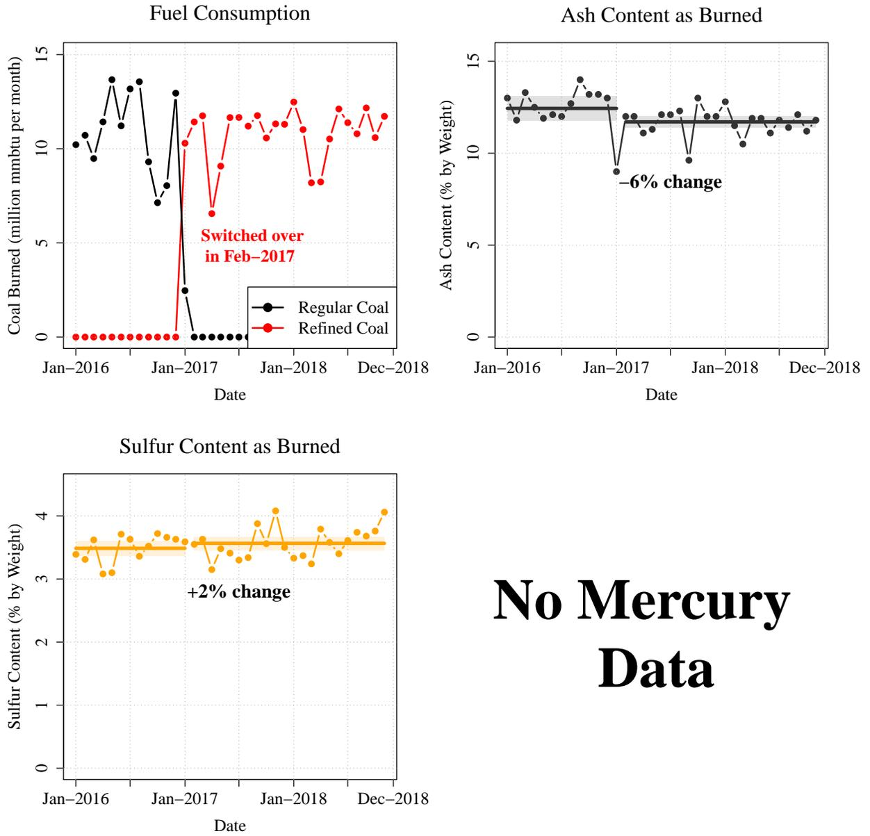
Figure A.5: Coal Characteristics for Plant 4 (in Figure 7)
