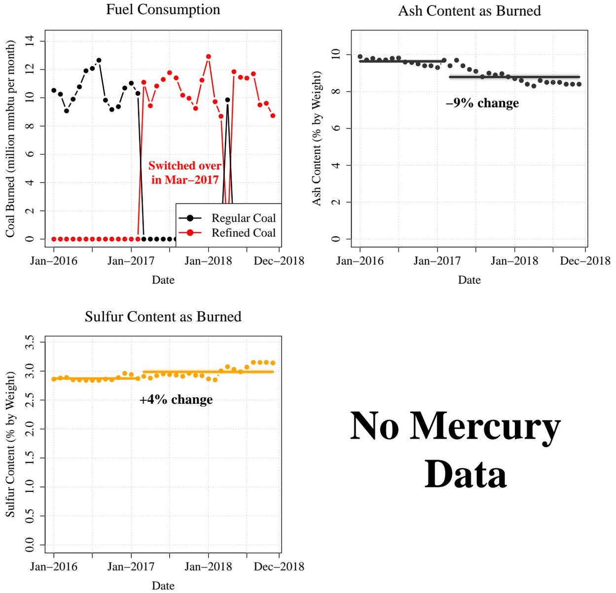
Figure A.4: Coal Characteristics for Plant 3 (in Figure 6)
