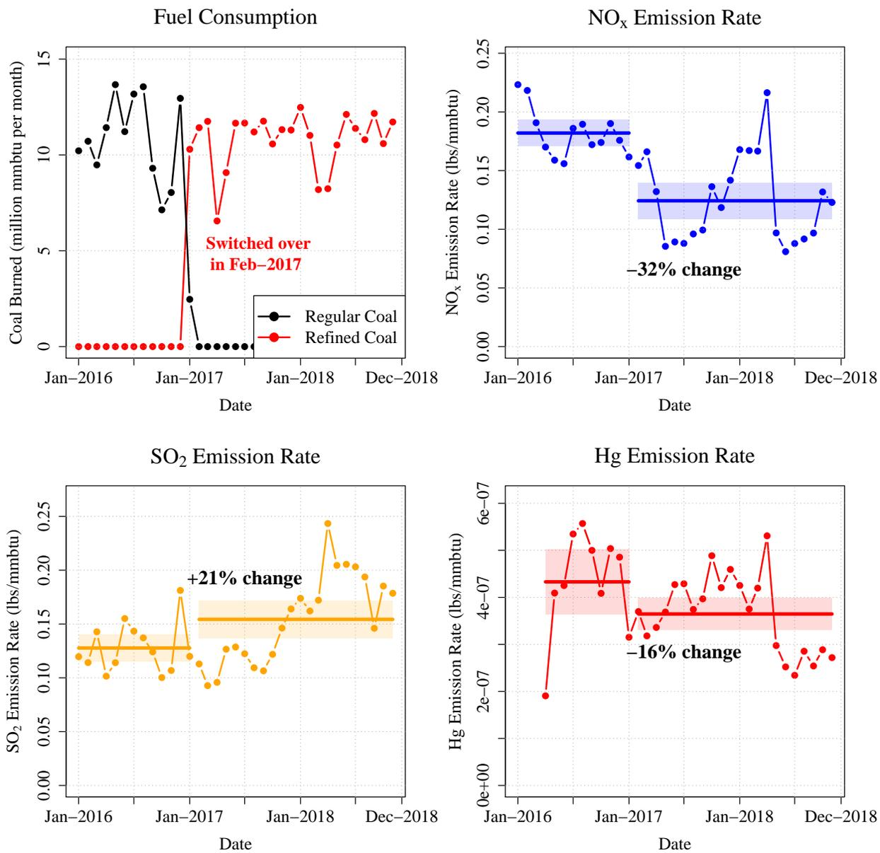
Figure 7: Fuel Consumption and Emission Rates: Plant 4
