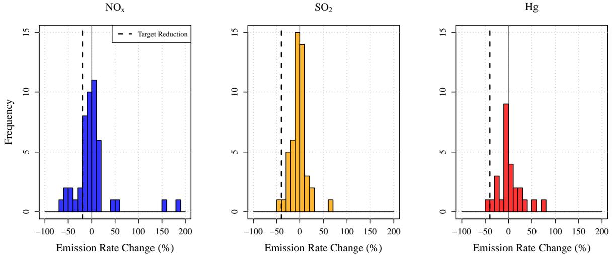
Figure 8: Histograms of Estimated Emission Rate Reductions for Boilers with Sufficient Data
