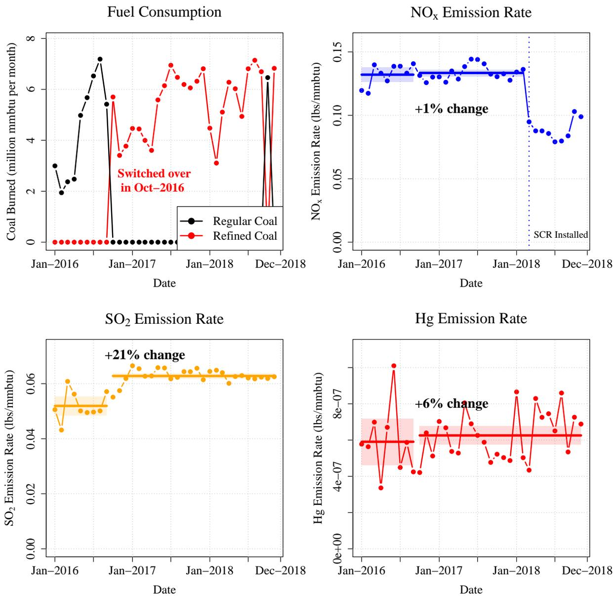
Figure 5: Fuel Consumption and Emission Rates: Plant 2
