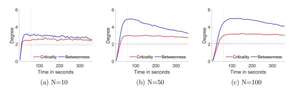
Figure 15: Mean degree (dotted lines represent the expected values predicted by the computer simulations)
